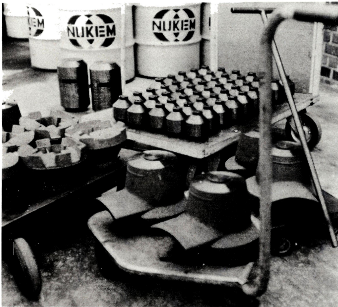
Depleted uranium metal can be cast into any desired shape
